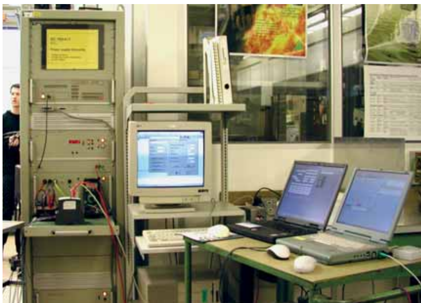
Measurement of the behaviour of the devices in voltage dips, brief interruptions or voltage fluctuations of the power supply
