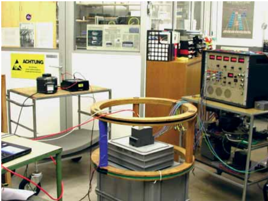
Determination of device behaviour under the influence of a magnetic external field generated by a Helmholtz coil
